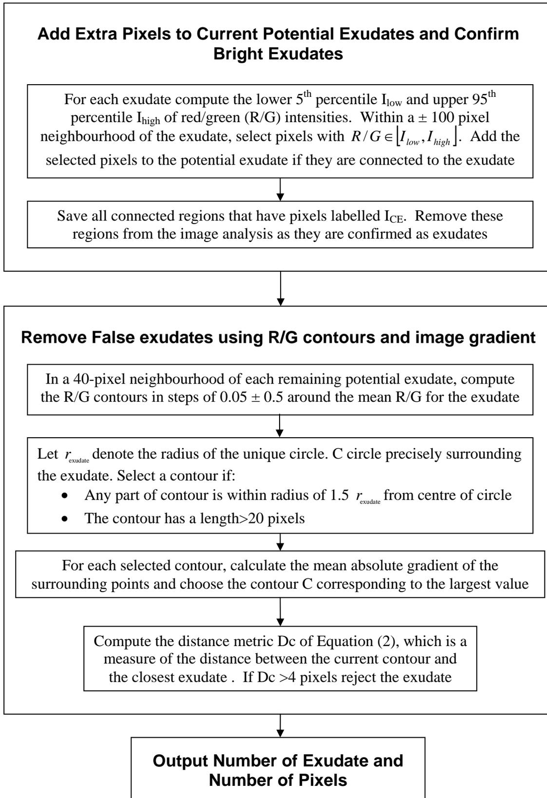
Figure 7: Algorithm for detecting exudates
