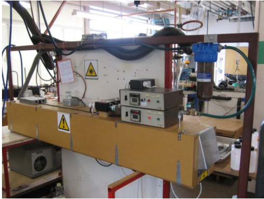
Figure 3.7. Accelerated UV weathering system
