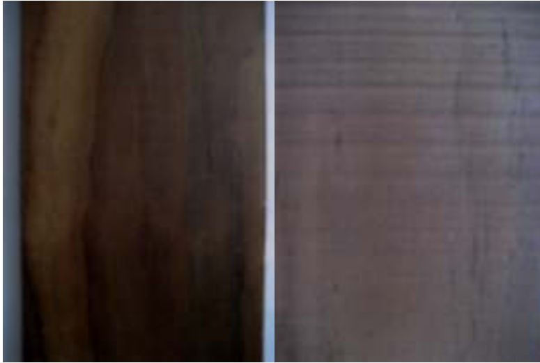
Figure 4.7. Wood colour at surface (left) and core (right) of the specimen treated at 210°C
