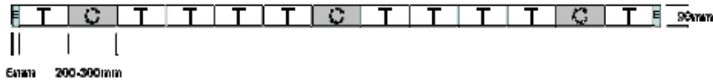
Figure 3.2. General cutting pattern of the specimens from a board where: E represents the trimmed ends; T represents the treatment specimens and C the control (untreated).
