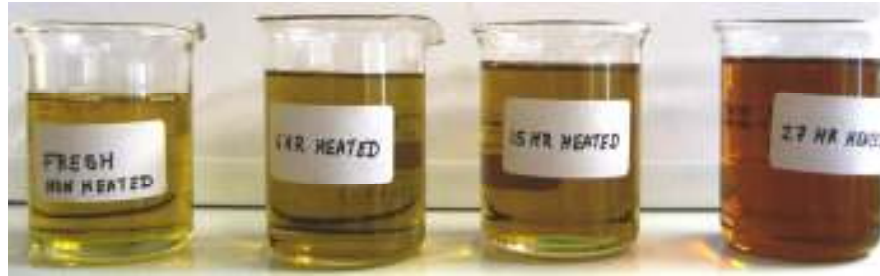
Figure. 7.2. Colour change in linseed oil with prolonged heating, from left to right showing fresh oil, and that heated for different hrs
