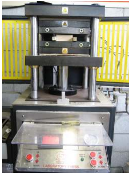
Figure 5.1. Laboratory press used for TMC of wood specimens
