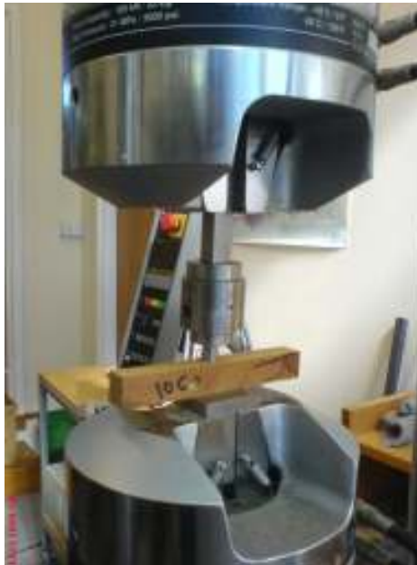
Figure 3.6. Janka indentation test at the MTS machine
