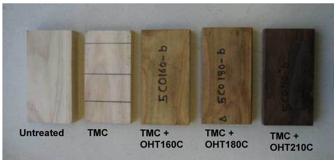
Figure 5.2. Colour of wood in TMC wood and TMC+OHT wood treated at different temperatures
