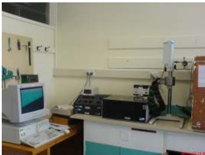
Figure 7.1. Haake viscometer used for measurement of viscosity of linseed oil
