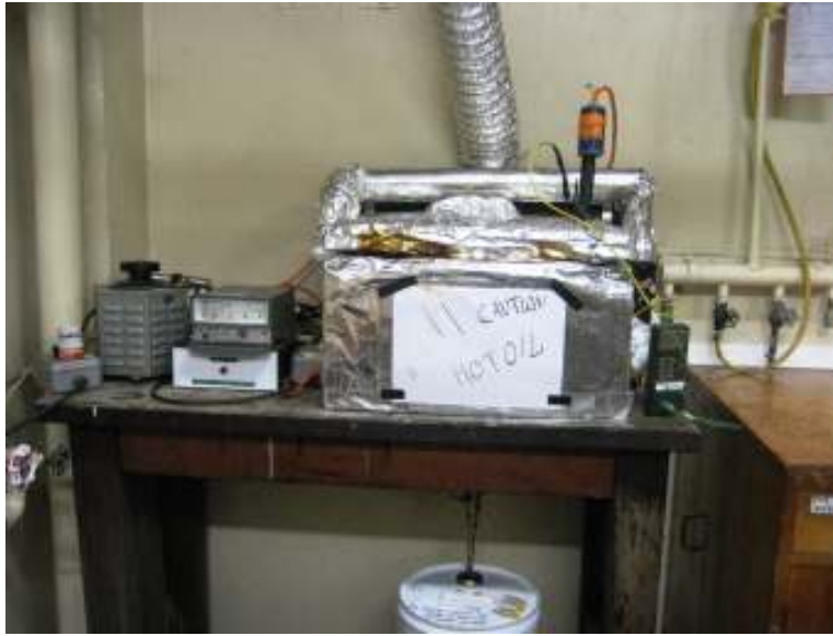
Figure 4.1. Oil bath used for heat-treatment.
