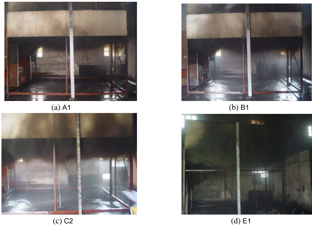
Figure 3. Smoke layer remains stable.
