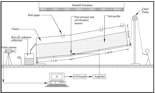
Figure 1. Schematic diagram illustrating the experimental set up.
