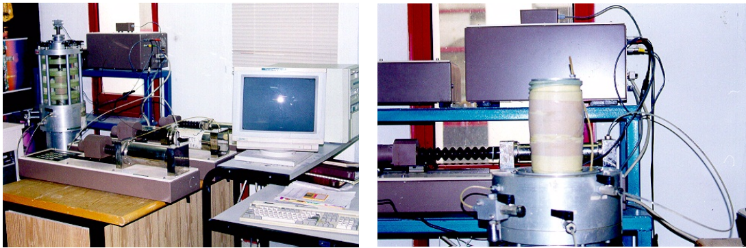
FIG.3. Photographic view of GDS triaxial testing system and failure pattern of a two layered reinforced soil specimen for CTC stress path for stress path tests
