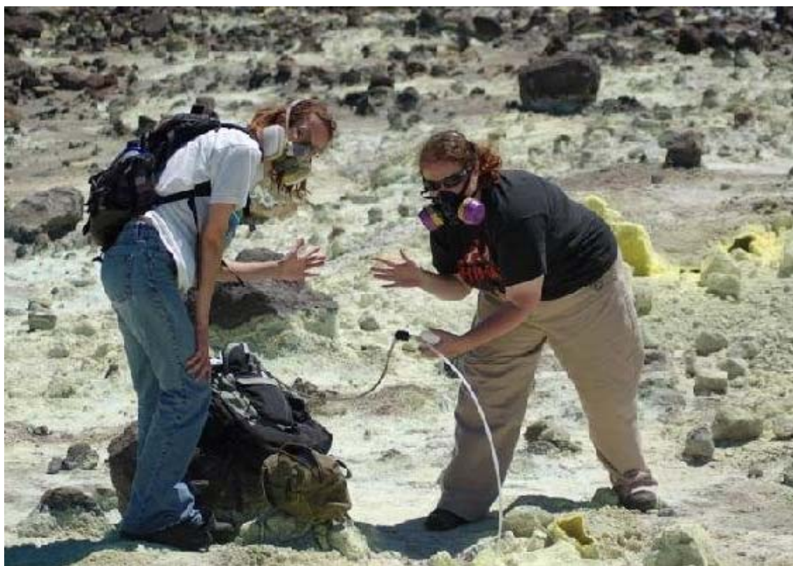
Figure 26 – Gas sampling using evacuated sample bottle at Kilauea. The vacuum inside the flask draws a sample into the bottle once the stopper is released, the sample is then analysed using a mass spectrometer in the laboratory (photo: Angela Doherty).
