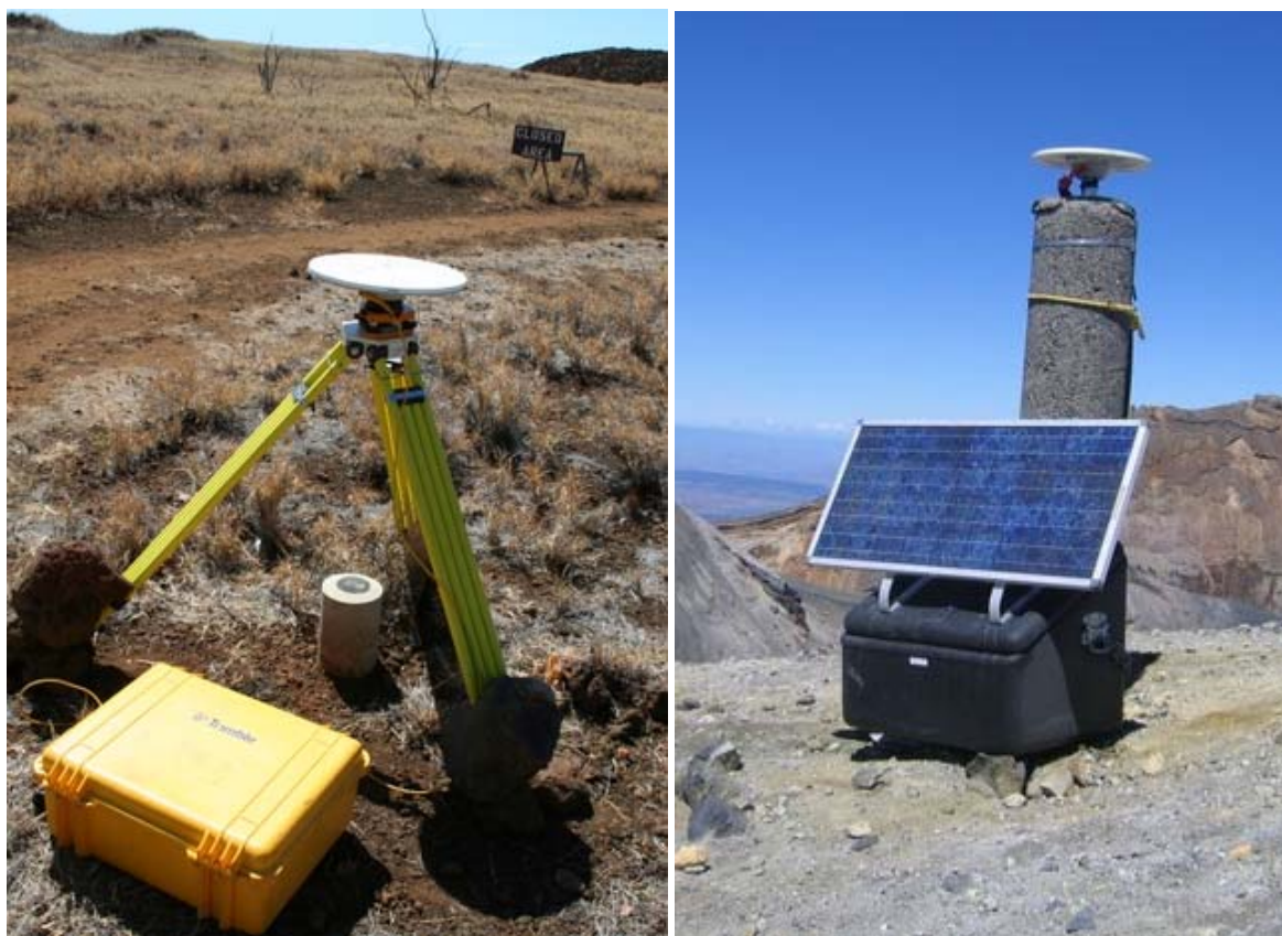
Figure 25 – GPS site in survey (left) and continuous (right) configuration (photos: Angela Doherty (left) and GNS 2009 (right)).
