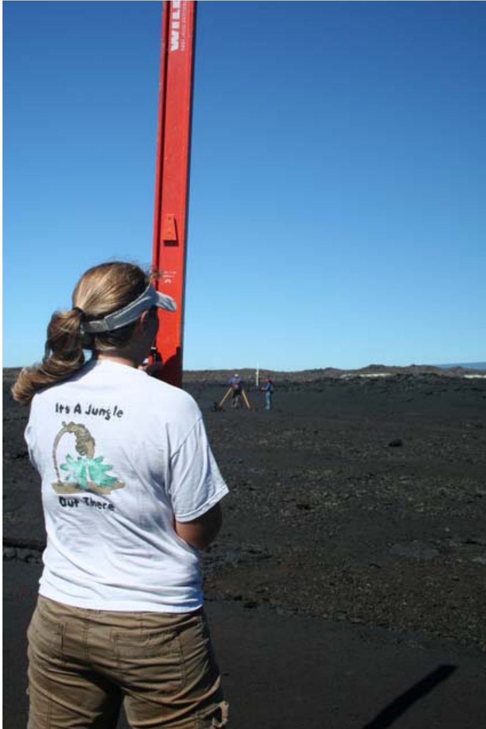
Figure 24 – Precise levelling campaign at the summit of Kilauea Volcano, Hawaii. Note the level in the centre of the image and second marker staff in the background (photo: Angela Doherty).
