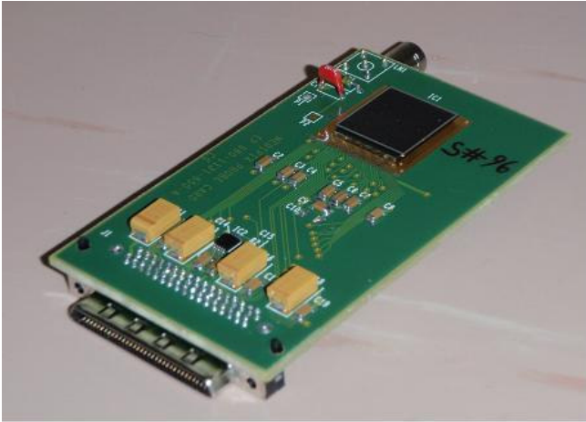
Figure 1. Photo of the Medipix2 detector with the semiconductor sensor layer bump bonded to the read-out chip.
