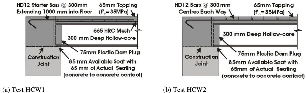
Figure 4 Connection details used in the two experimental tests
