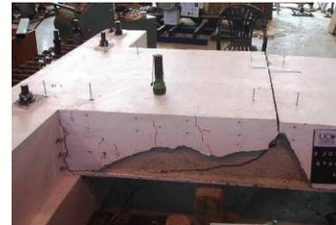
(c) South side after failure
