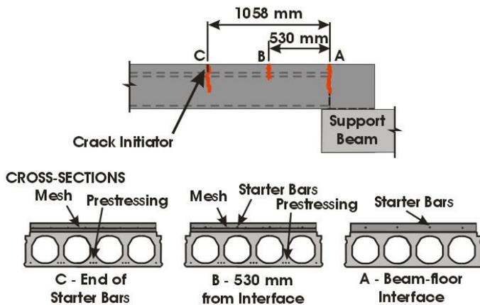
(a) Locations cracks formed in test specimen HCW1 during testing and cross-sections of the specimen at these locations
