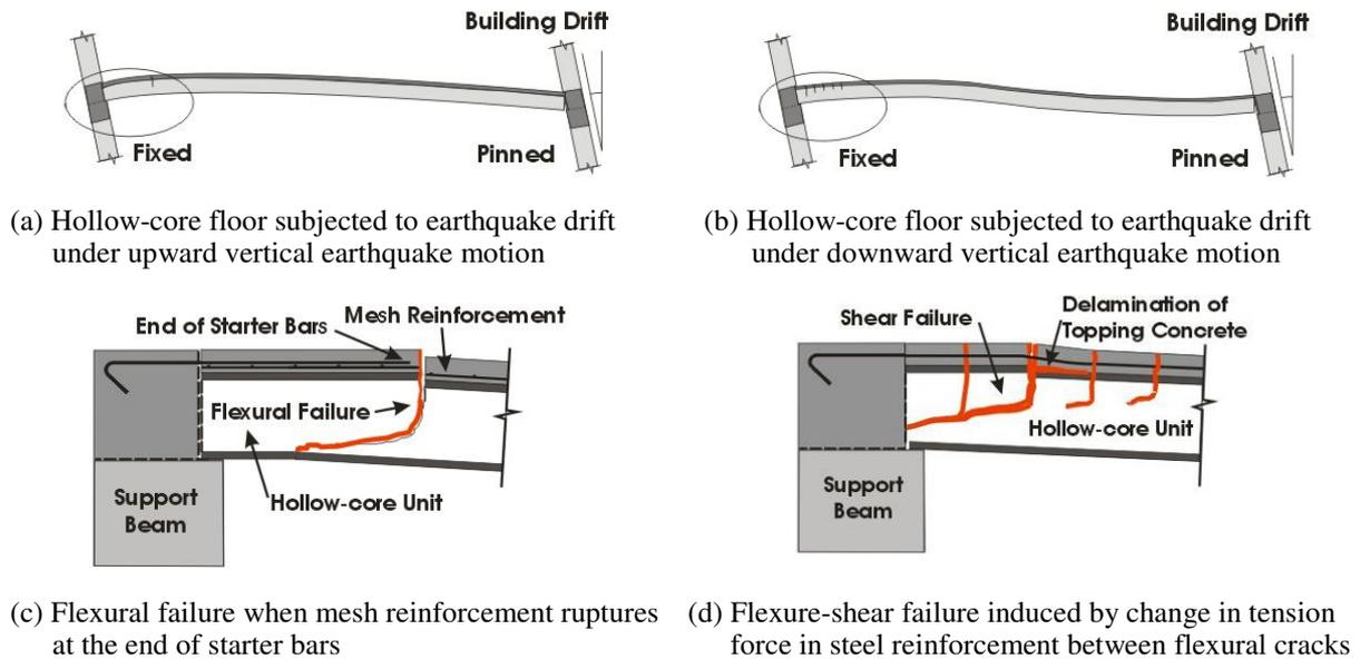
Figure 2 Potential failure modes of hollow-core flooring when subjected to negative bending moments
