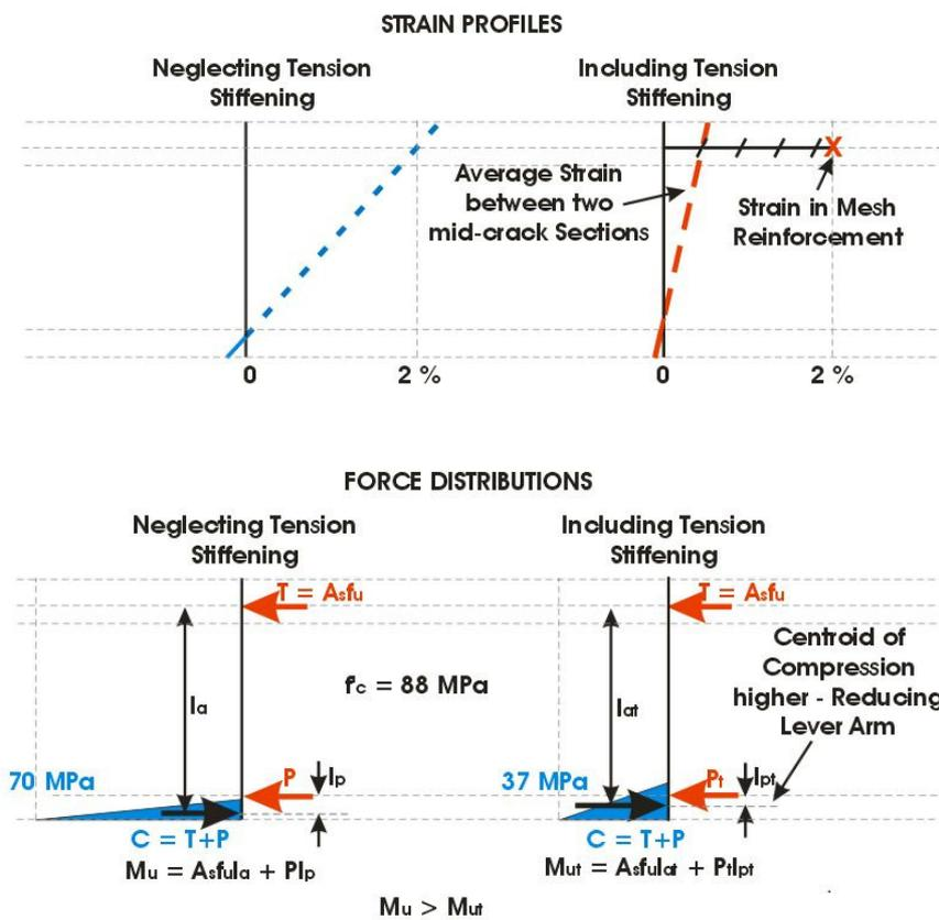
(b) Strains and forces in a prestressed hollow-core floor with topping containing mesh reinforcement
