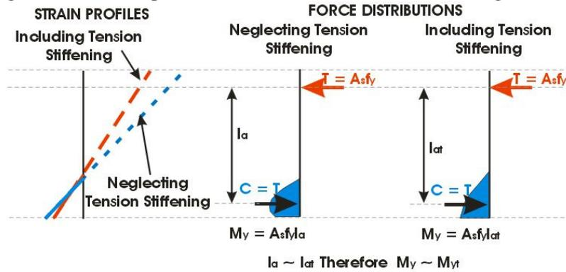
(a) Strains and forces in a typical reinforced concrete beam
