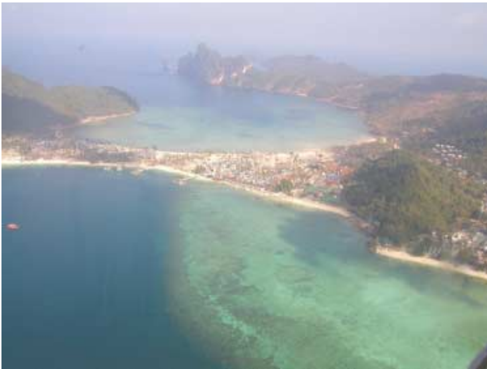
Figure 7. Phi Phi Island viewed from the air as the team approached by helicopter from the southeast. The tsunami wave traversed the sand-spit at depths of up to nine metres, first from the north and a few minutes later again from the south (Photo ED).
