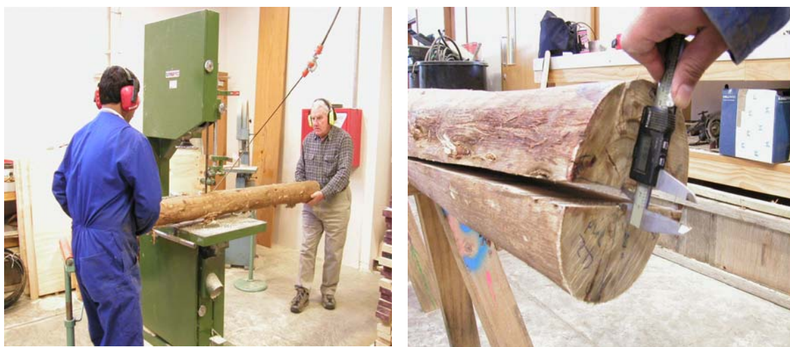
Figure 1: Log sawing and opening measurement
