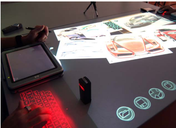
Fig. 5: The virtual keyboard from i.Tech and the virtual augmented control elements can be used respectively.
