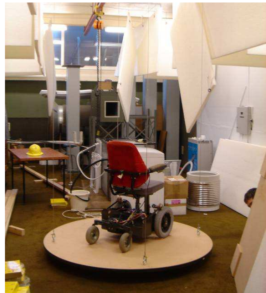
Fig. 8. Quadrifilar Pendulum setup for moment of inertia
