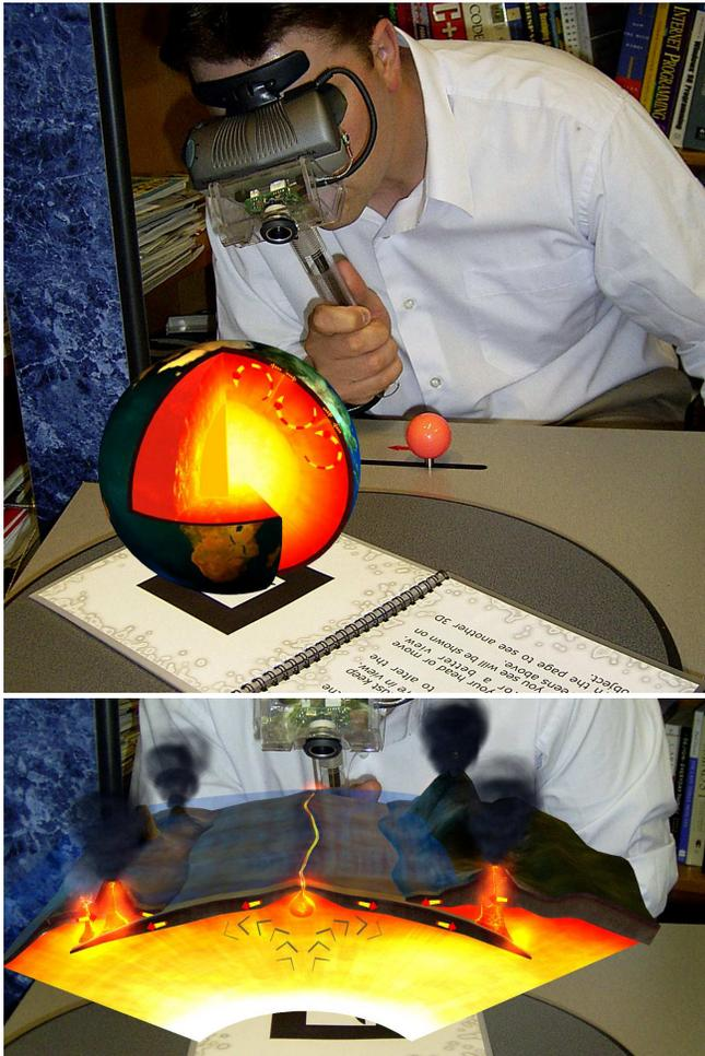
**Figure 5:** *Top:* The AR Volcano Kiosk in use. Note how the slider is being used to highlight the convection currents. *Bottom:* A page showing the use of dynamically-lit particle systems and pixel shaders for lava and water. The slider moves the tectonic plates.
