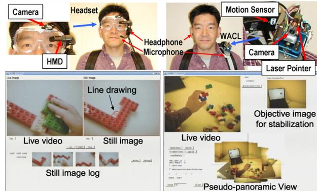
Figure 1: Headset interface and WACL interface.
