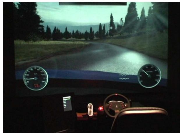
Figure 1. The car simulator consisting of a big projection screen, a steering wheel and a small LCD screen.
