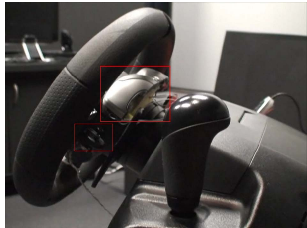
Figure 2. The interaction device consisting of a scrolling wheel and two buttons (left and right).
