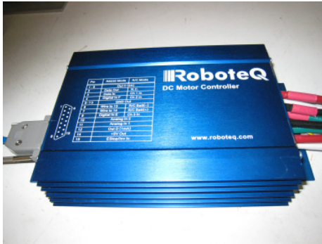
Fig. 7. The controller for both horizontal and vertical thrusters.
