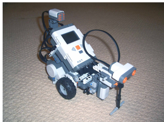
Fig. 5. Lego Mindstorms NXT robot in the Tribot configuration.
