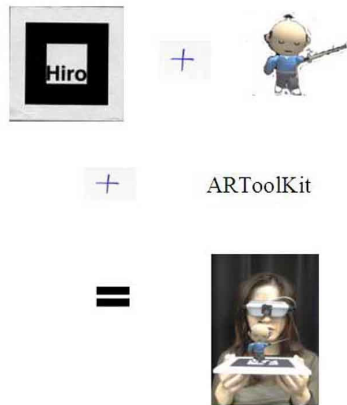
Fig. 2. ARToolKit tracks a fiducial marker and aligns an object in AR that appears registered in the real world.
