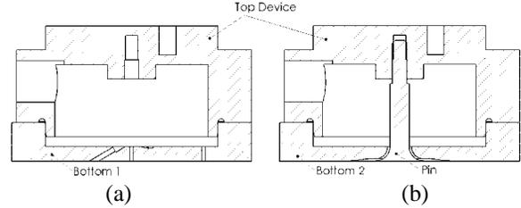
Fig. 9. Cross-section of Experimental Device with mounted Bottom 1 (a) and Bottom 2 (b)
