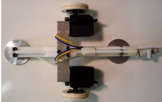
Fig. 13. Top view of the wall climbing robot with two Bernoulli pads and two wheels.
