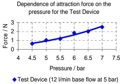
Fig. 8. Maximum adhesion force at a certain pressure
