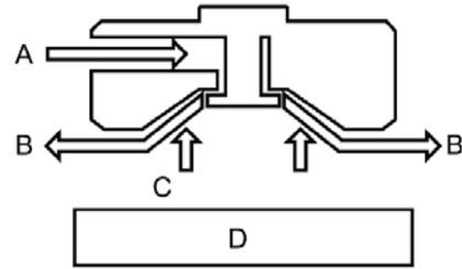
Fig. 2. Functional principle of NCT. A: Supplied pressure, B: Outlet air stream, C: Lifting force, D: Object.
