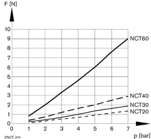
Fig. 3. Lifting force  $F$  at pressure  $p$  for different NCT devices
