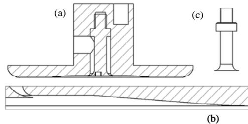
Fig. 10. Cross-sections of (a) the Bernoulli pad, (b) detail of the undercut with the angled ramp, and (c) the pin.
