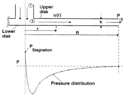
Fig. 1. Radial pressure distribution on a disk
