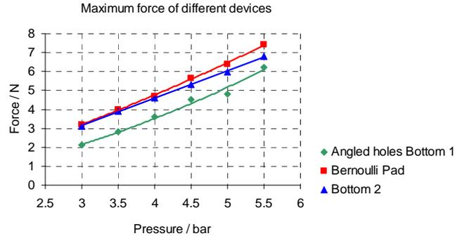
Fig. 11. Maximum force of different device with flow rates.
