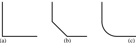
Fig. 5. Edge designs for the outer diameter of the pad: (a) sharp edge, (b) angled edge, and (c) rounded edge
