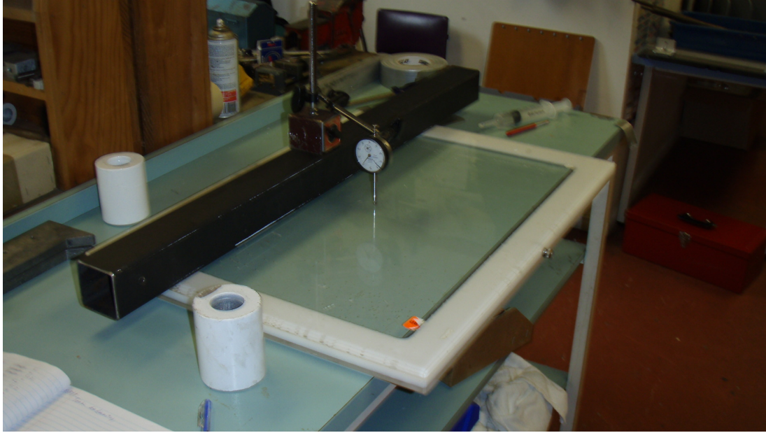
Figure 3.6 DTI on flood phantom to measure relative deformation
