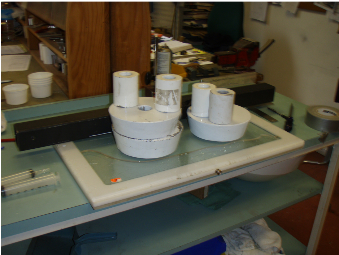
Figure 3.7 Weights placed on phantom to measure deformation. The DTI is obscured from view by the weights.
