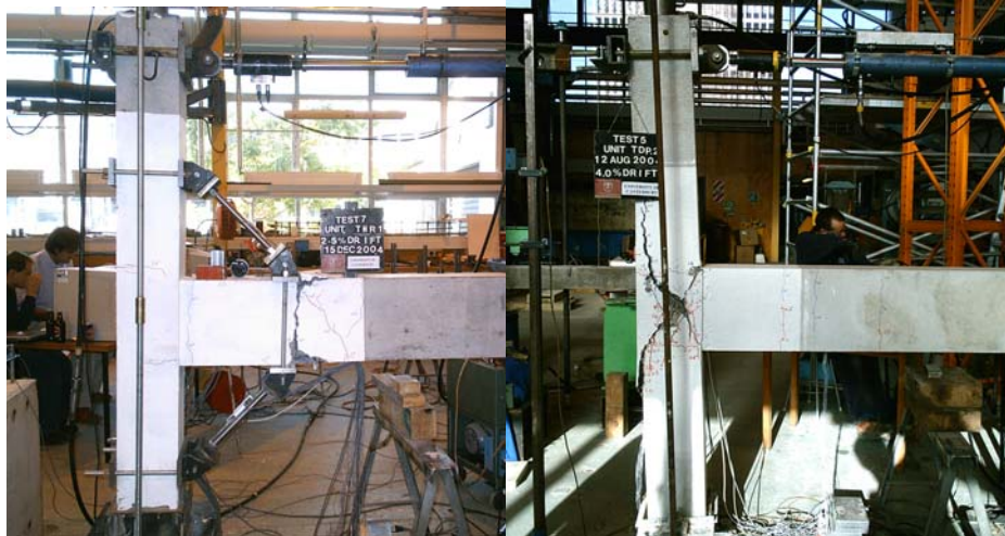
Figure 9: Comparison of Observed Damage in the Retrofitted (THR1, left) and As-built (TDP2, right) Specimens
