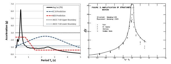
Figure 2: Comparison (left) of predicted floor acceleration response spectra at top level of an 8-storey RC wall building (from Sullivan et al. 2013) and (right) dynamic amplification factors (ratio of acceleration demand on a component to peak floor acceleration demand) from Biggs (1971).
