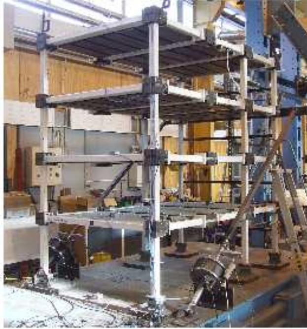
Figure 2. Photograph of test structure on the shake table with the devices installed.
