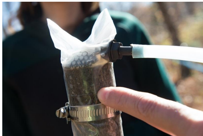
Figure 3. A picture of the sap-collection device used to extract sap from the top of maple saplings. Picture used with permission from Sally McCay, Photographer for UVM Photo.
