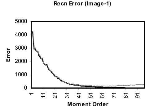
Fig. 9. Plot of image-1 reconstruction error with moments computed using (18)–(22). The dotted line shows the change in error when noise is added to the input image.
