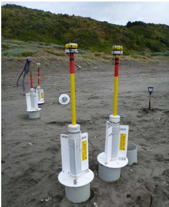
Figure 2 Photo showing the design of the GPS drifters used at Ngarunui Beach.
