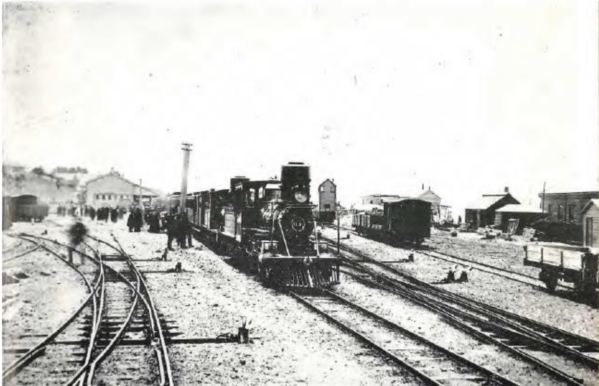
Figure 27. Excursion train arriving at Timaru, 1880. The leading locomotive is an American-built K-class, assisted by a British-built J-class. Photograph: Pierre, p. 101.
