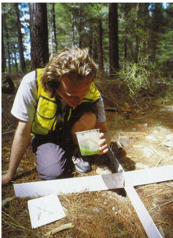
Figure 2.2 Pitfall trap design. I am holding the polypropylene plastic container that is buried to ground level beneath the junction of the two white plastic guide panels when the trap is operational. An ice cream container lid (lower corner of photo) is used as a rain cover and is held in place over the guide panels above the plastic container by wire pegs. Photo by Kennedy Warne.
