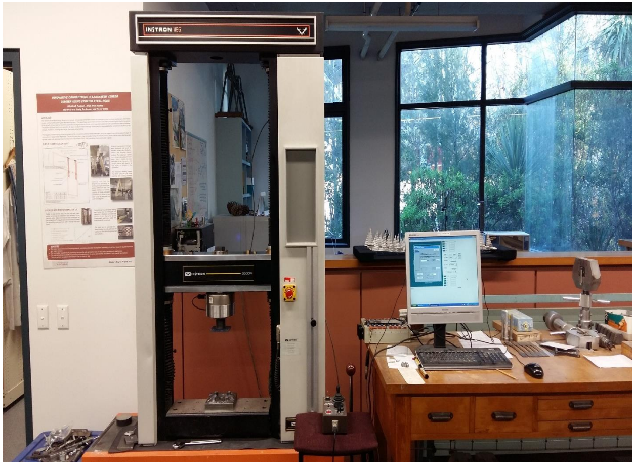
Figure 3-45: Instron machine with data recording software and crosshead speed controller (Model Structures Laboratory, University of Canterbury)
