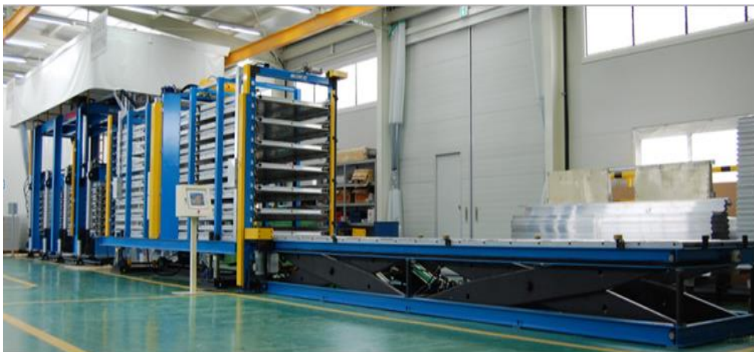
Figure 2-21: Multi-opening vertical hot press (Trade Belt)
