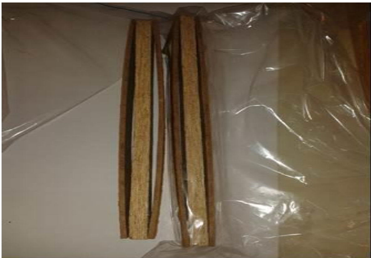
Figure 1-3: Comparison of bowing between slices kept in ambient conditions and those wrapped in plastic bags
