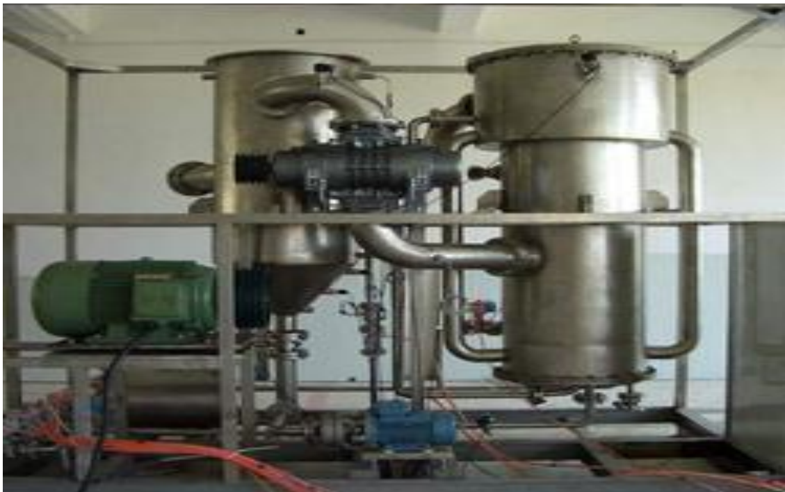
Figure 3-37: Natural and forced circulation dryer (After Espoir Engineering Pvt. Ltd.)
