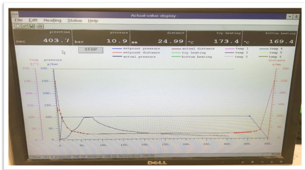
Figure 3-38: Data logging during hot pressing for board A1
