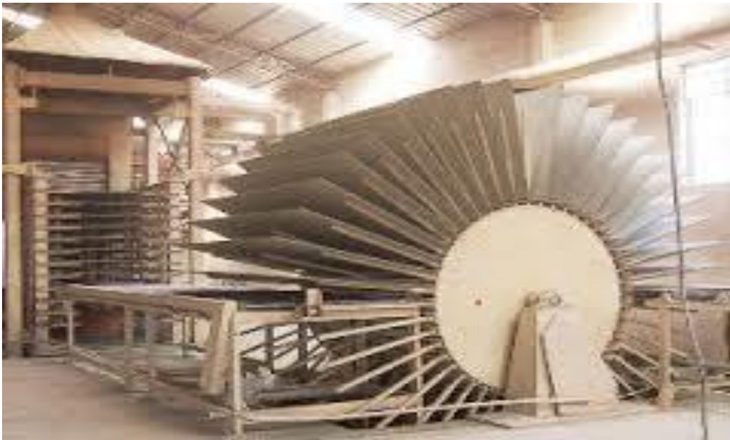
Figure 2-22: Cooler for hot pressed boards (Shandong Tengfei Mechanical and Electrical Technology Co., Ltd.)
