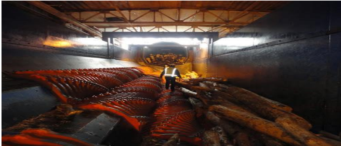
Figure 2-17: Industrial size log debarker (IEM Ltd.)
