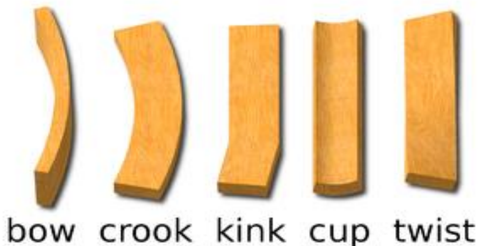
Figure 1-2: Types of warping observed in wood panels (after Wikipedia)
