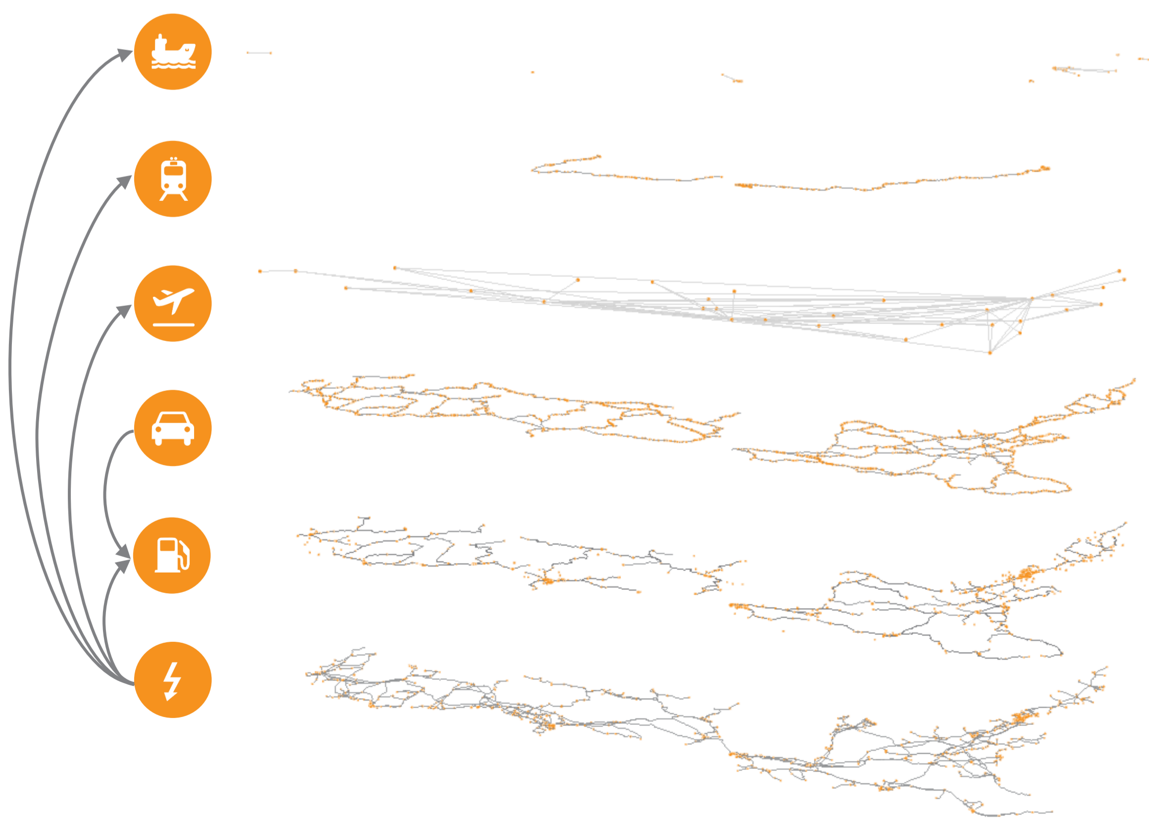
Fig. 1. Network overviews of selected transportation and electricity infrastructures used with arrows indicating service flow for normal operation.
