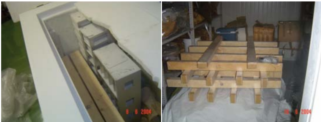
Figure 2-2. Freezers used for conditioning to -71°(left) and -20°(right), boards are tightly wrapped with cling film
