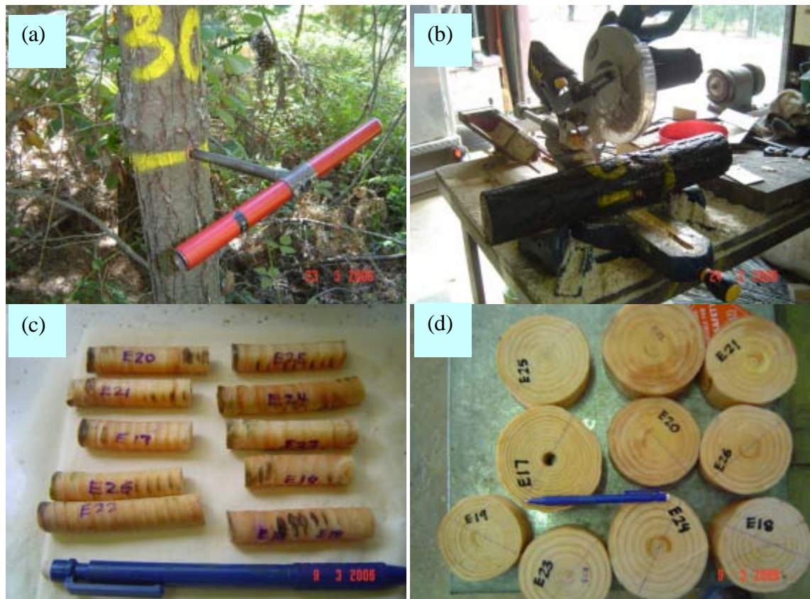
Figure 4-2. Details of the second set of samples collected in summer 2006 for further validation of 12 mm cores: a) manual borer; b) dropsaw for extraction of disk from billets; c) batch of 12 mm pith-to-bark cores, and the corresponding (paired) dropsaw disks (d)
