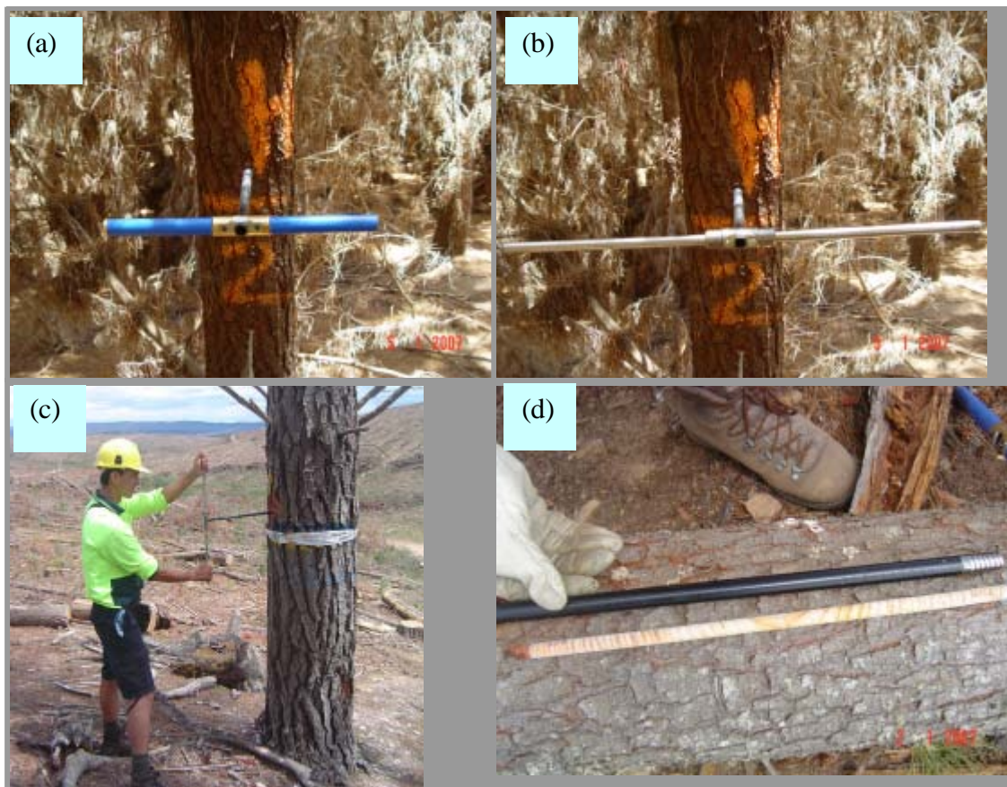
Figure 4-3. Procedures for extraction of 12 mm cores showing: a) Initial engaging and coring using normal handle; b) custom-made steel handle; c) coring a large mature tree; d) damage-free and smooth bark-to-bark core obtained from a large tree
