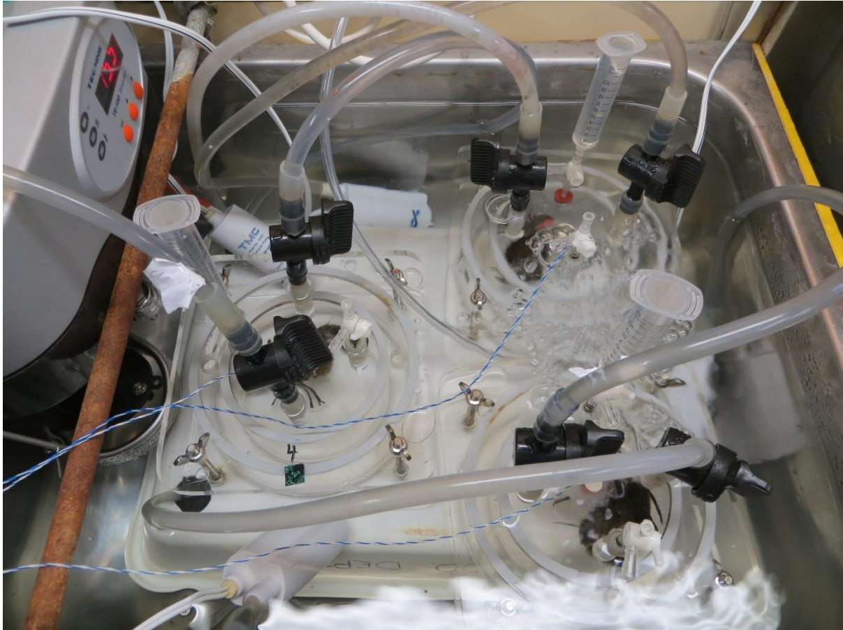
Figure 2.1: Photograph showing the respirometer set up in the water bath.
