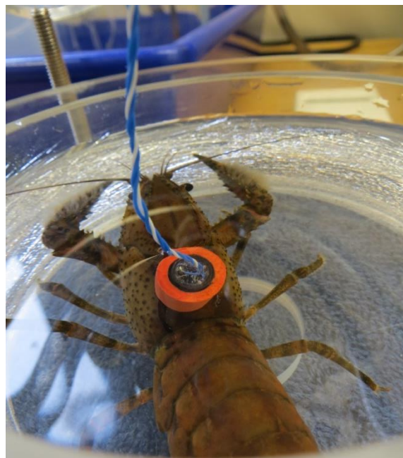
Figure 2.3: Photograph showing the IR sensor slotted into the rubber bung that was glued onto the carapace of the crayfish.
