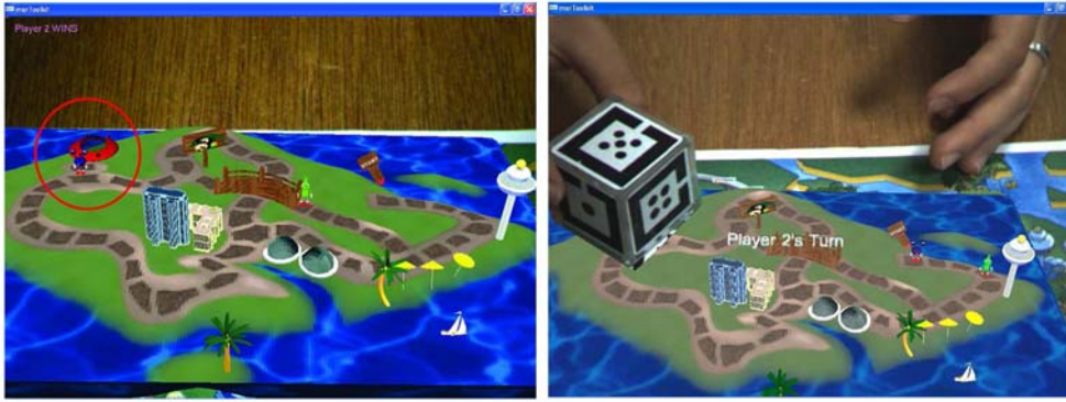
Figure 2.3: Jumanji Singapore: Using an AR marker cube for a range of tangible interactions (Image courtesy of Adrian David Cheok, Mixed Reality Lab, National University of Singapore)
