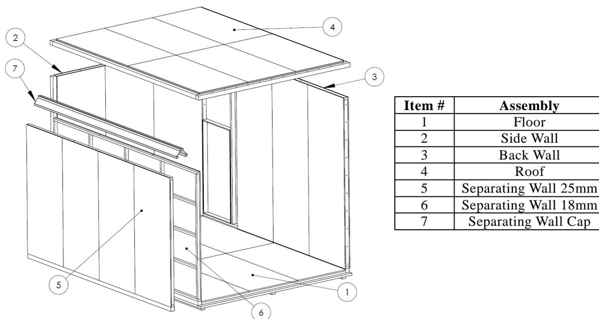
Figure 2 - Exploded view of one of the two identical rooms to be constructed for the CAC test facility.
