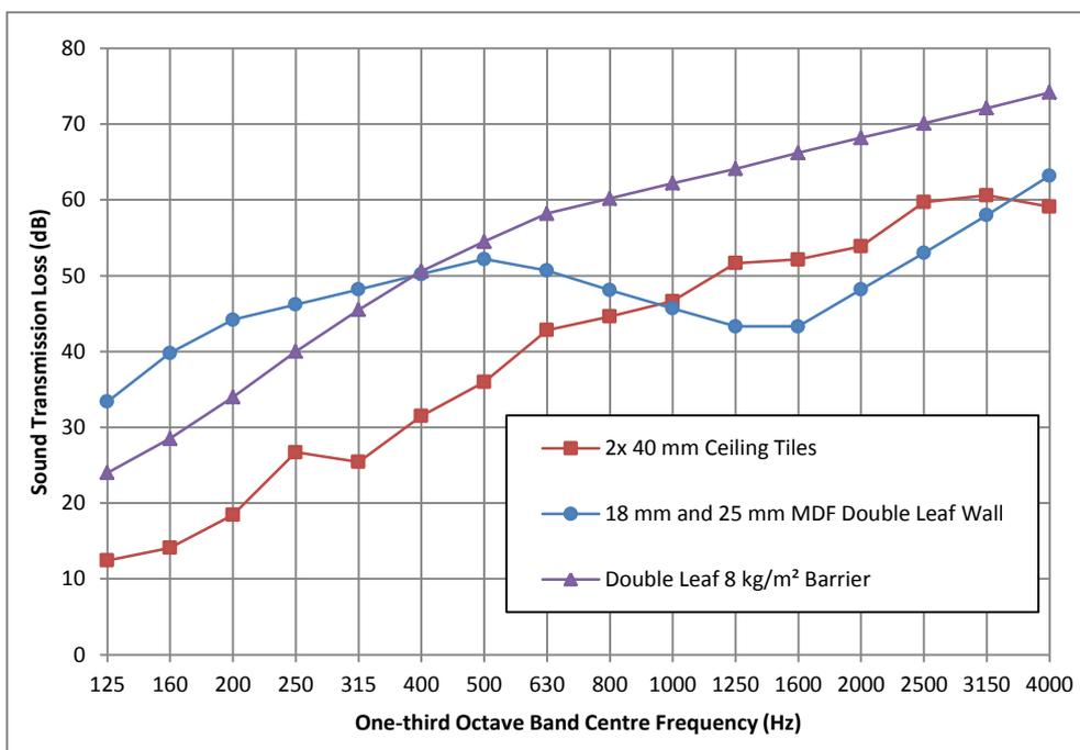
Figure 6 – Estimated sound transmission loss of two walls compared to estimated sound transmission loss of ceiling system.
