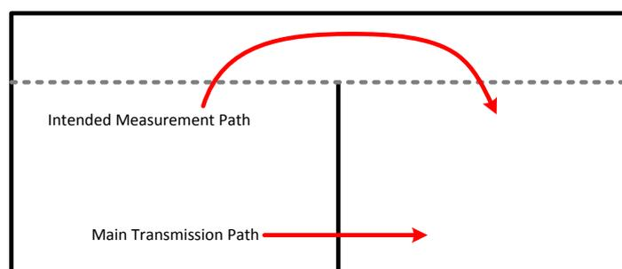
Figure 4 – Main sound transmission paths present in the test facility.
