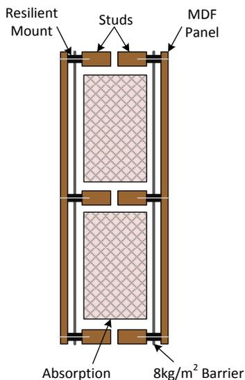
Figure 7 – Proposed separating wall design.
