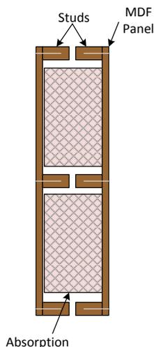
Figure 5 – Initial separating wall design.
