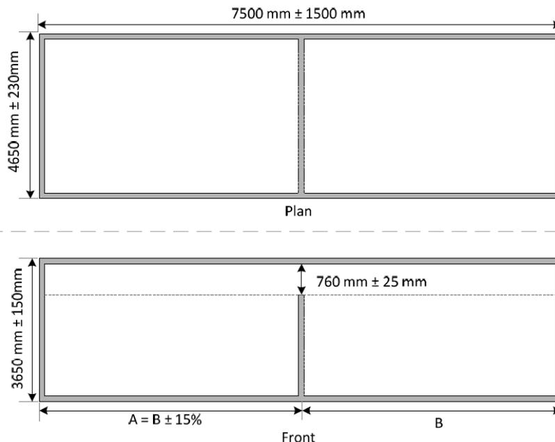
Figure 1 - Dimensions of test facility required by ASTM E1414
