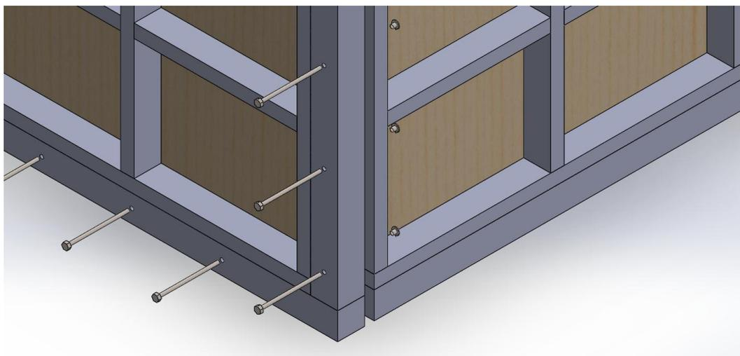
Figure 8 - The test facility bolt and T-nut construction method. Note: The outer leaves of the wall are hidden so the T-nut locations are visible
