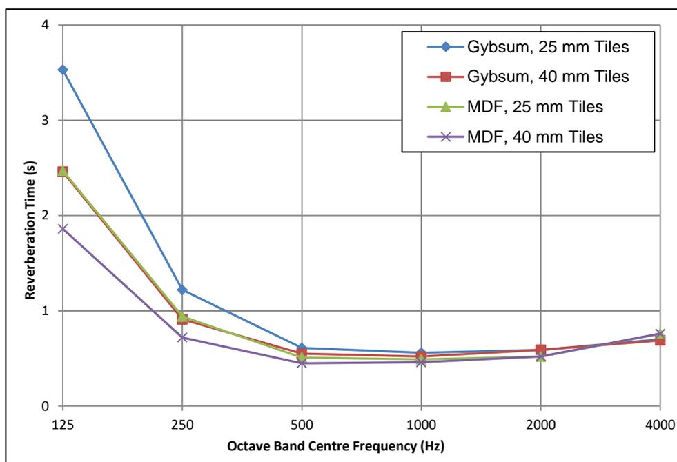
Figure 3 – Predicted reverberation times, gypsum vs. MDF, with the two ceiling tiles modelled
