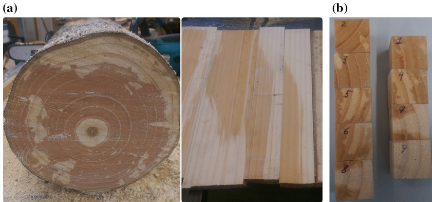
Fig. 1 a P. radiata log from Owen River forest (Nelson region) with the internally developed dry patches and b the blocks of various dryness, showing the four right hand blocks selected for EC measurements on partially dried wood
