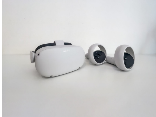
FIGURE 5.1: Oculus Quest 2. The system is battery powered and can be used without a connection to a computer. Image by Maximilian Prandstätter on Flickr - CC BY 2.0 2
