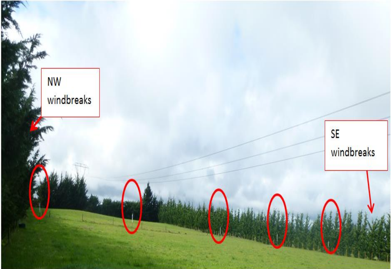
Figure 3-14. Photograph showing wind logger settings perpendicular to both windbreaks when viewed from the south (red circles represent the wind loggers).
