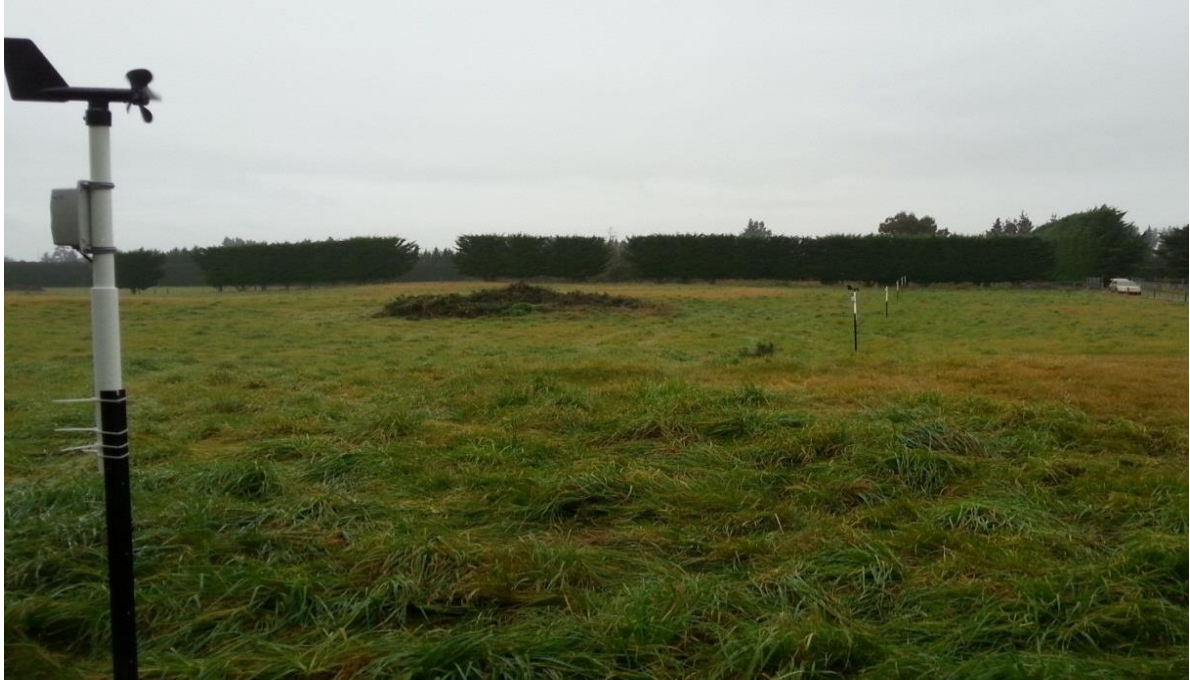
Figure 3-17. Photo showing the set-up of wind loggers perpendicular to the eastern windbreaks at Site 2 when viewed from the west.
