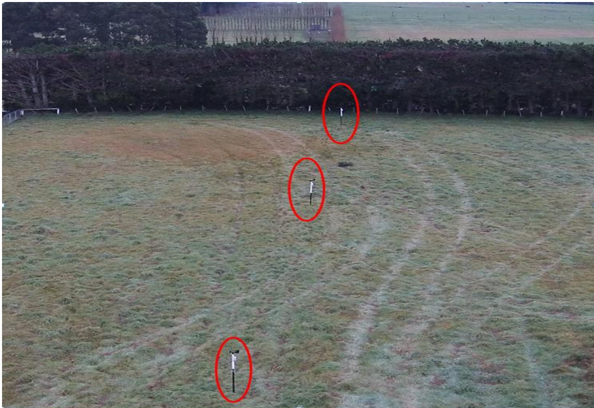
Figure 3-18. Photo showing the set-up of wind loggers perpendicular to the western windbreak at Site 2 when viewed from the east. Red circles indicate the wind loggers.
