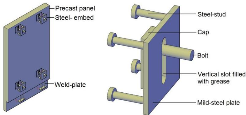
Figure 1. Precast panel with rocking connections (left) and steel-embed with vertical slot (right) [8].
