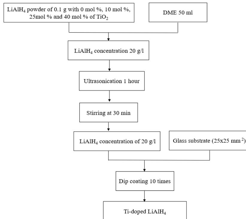
**Figure 1.** The process of Ti-doped LiAlH<sub>4</sub> thin film preparation under the controlled humidity and inert nitrogen atmosphere.
