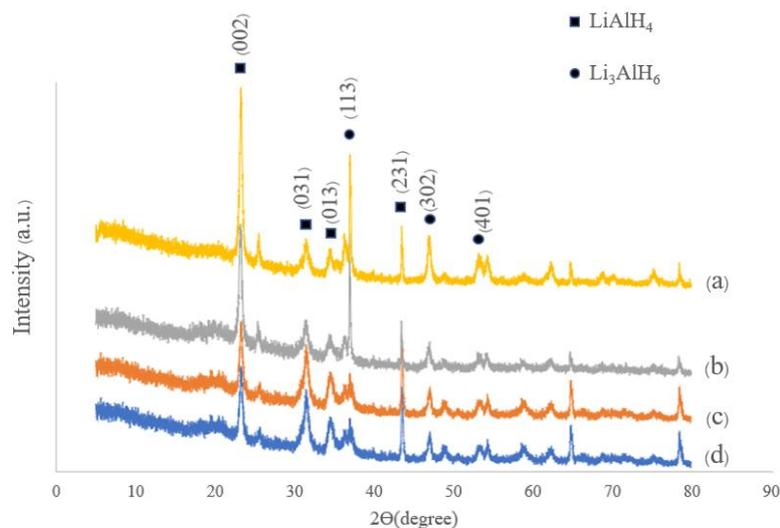
**Figure 2.** XRD patterns of the deposited Ti-doped  $\text{LiAlH}_4$  thin film at the  $\text{LiAlH}_4$  concentration of 20 g/l and  $\text{TiO}_2$  concentrations of (a) 0 mol%, (b) 10 mol%, (c) 25 mol% and (d) 40 mol%.
