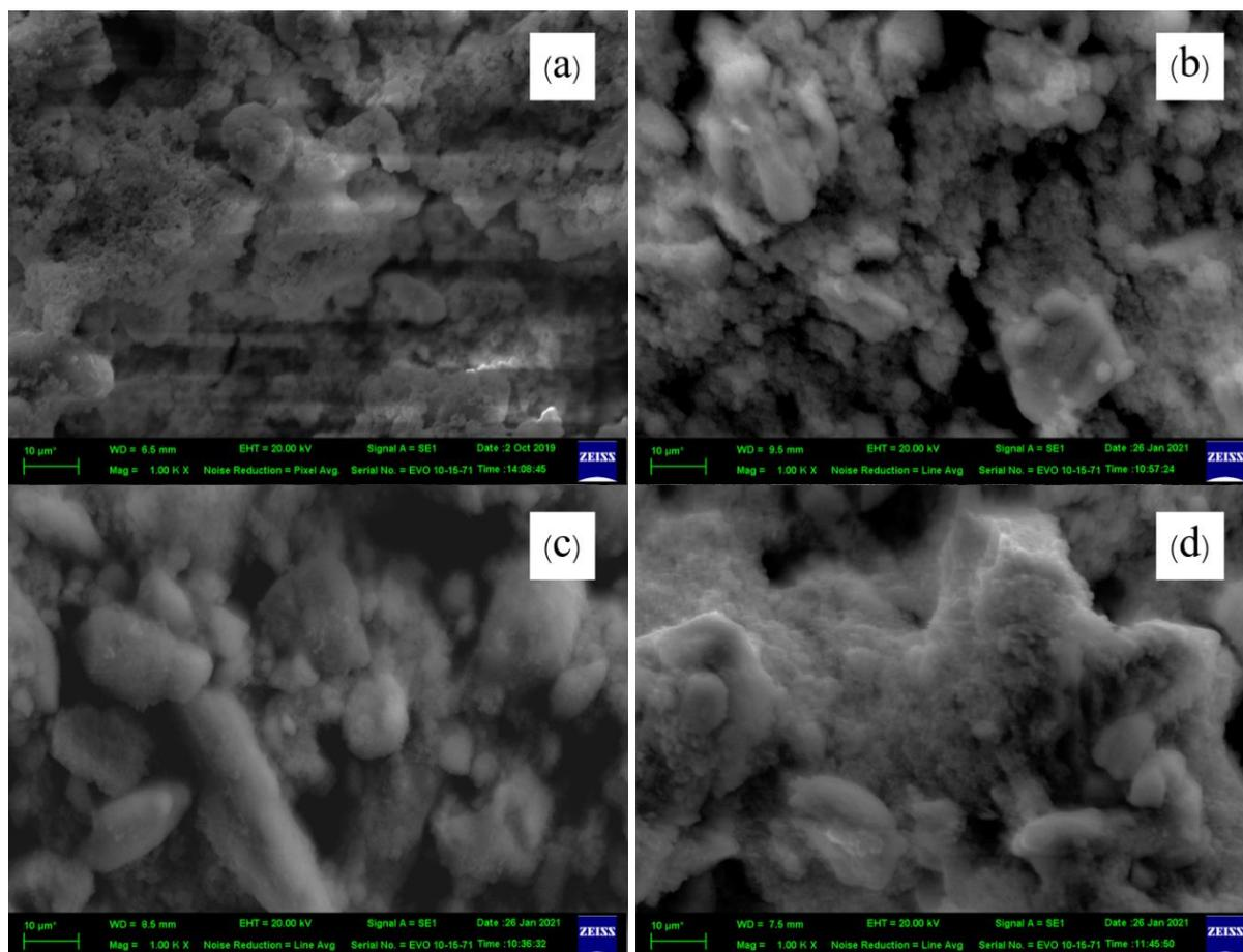
**Figure 3.** SEM images (1000x) of  $\text{LiAlH}_4$  concentration of 20 g/l with the different  $\text{TiO}_2$  concentrations: (a) 0 mol%, (b) 10 mol%, (c) 25 mol% and (d) 40 mol%.
