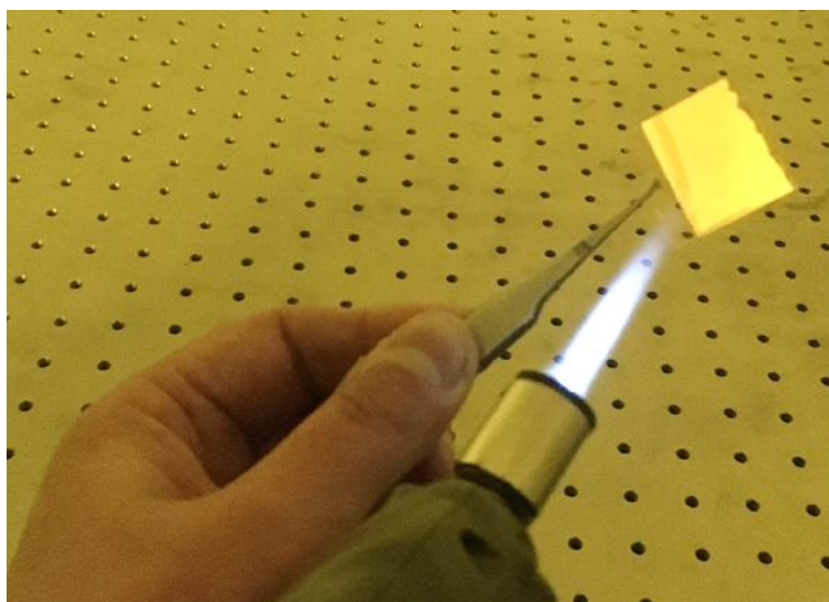
Figure 3.7. Photograph of the flame annealing procedure, where the slide with the gold film to be annealed is held in air by a pair of tweezers, while a flame is directed at the surface for 3 seconds and then left to cool down for 7 seconds. This process was repeated 3 times consecutively to yield the desired surface.
