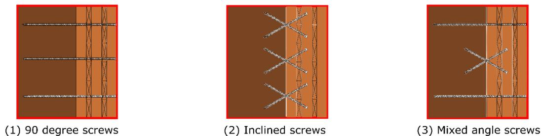
Fig. 4 - Orthogonal joint screwed connection options
