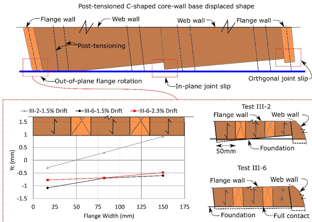
Fig.17 - Core-wall out-of-plane behaviour
