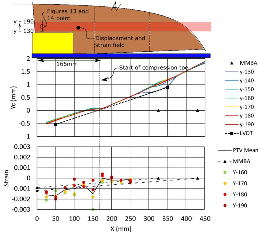
Fig.12 - Test I-2- Displacement and strain distribution with comparison to MMBA
