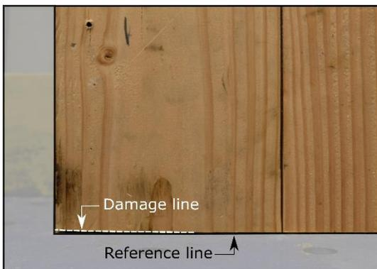
Fig. 8 - Wall 2 toe after Phase II
