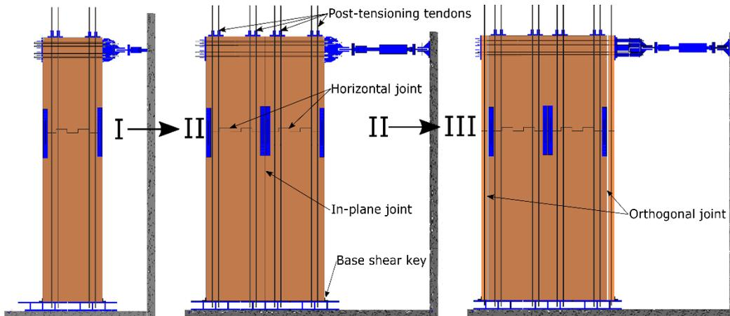
Fig. 3 - Post-tensioned CLT wall testing programme
