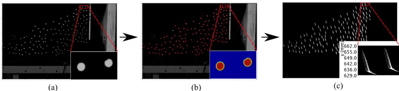
Fig. 6 - Particle identification: (a) Image filtering, (b) particle identification, (c) particle path
