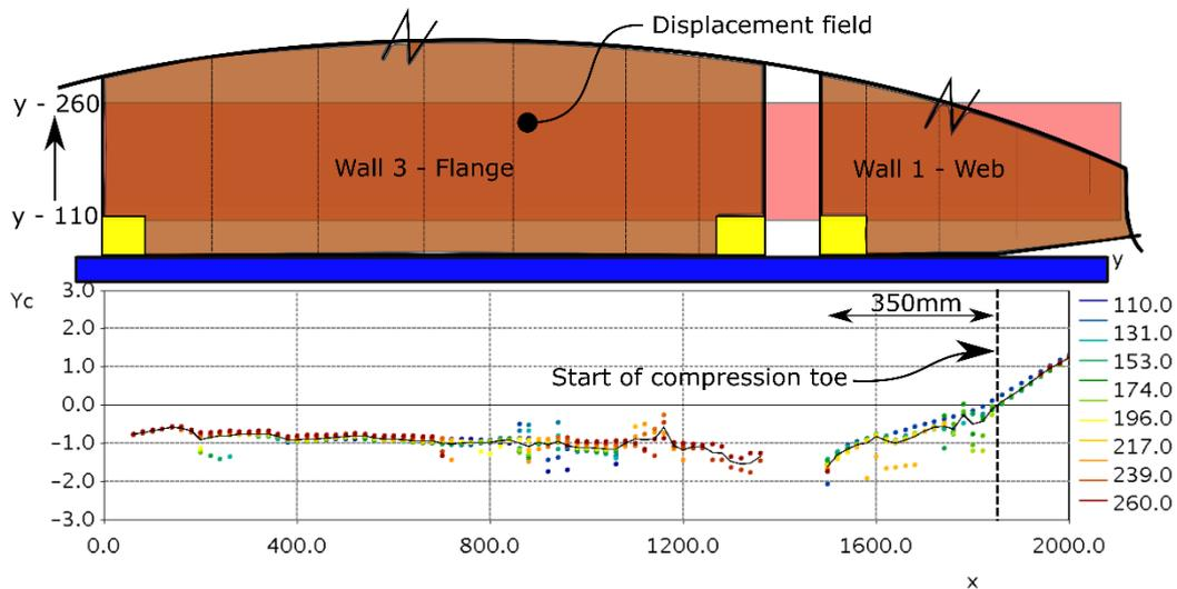
Fig. 16 - Test III-2 compression toe displacement at 1.5% drift
