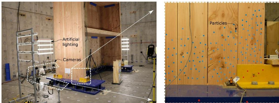
Fig. 5 - PTT setup at core-wall base: general setup with image from a single camera
