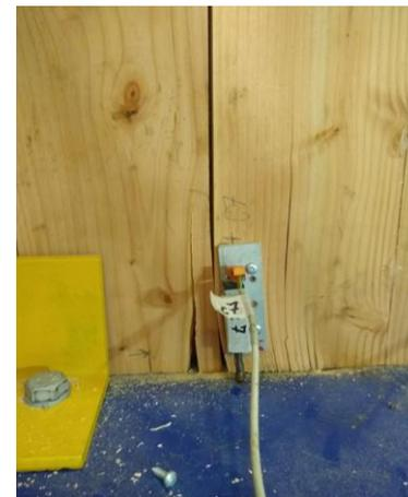
Fig.11 - Wall 2 compression failure at LVDT
