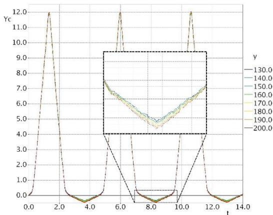
Fig.13 - Test I-2 displacement at 0.9% drift
