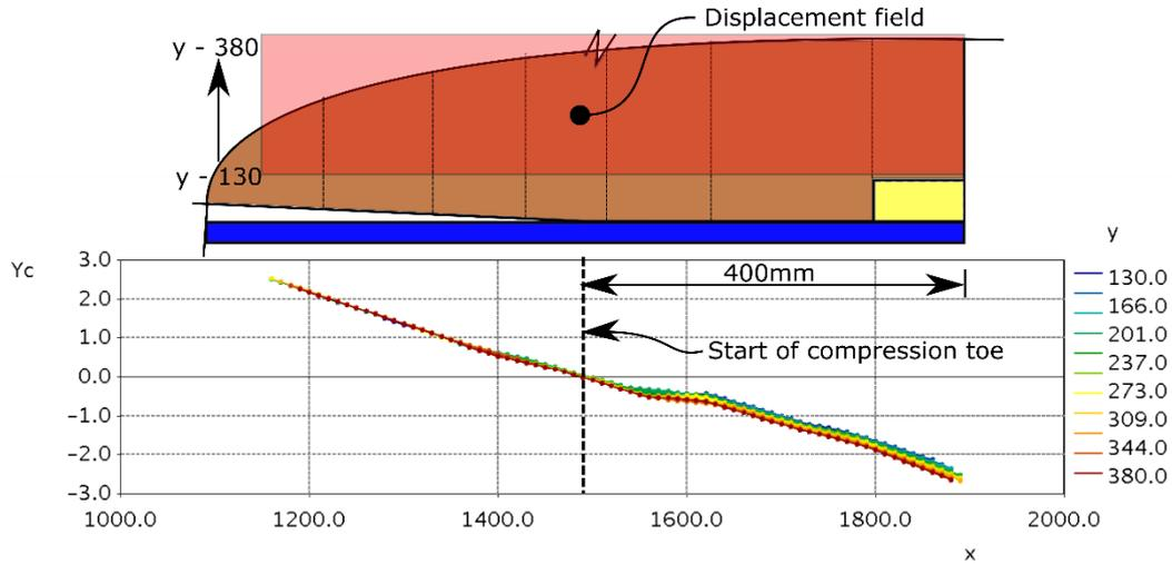
Fig. 15 - Test II-3 compression toe displacement at 1.2% drift
