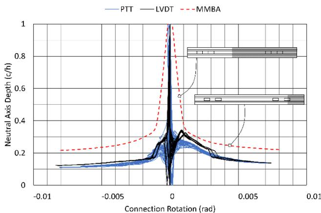
Fig.10 - Test I-2 - Neutral axis depth comparison
