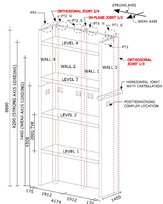
Fig. 2 - Core-wall specimen isometric
