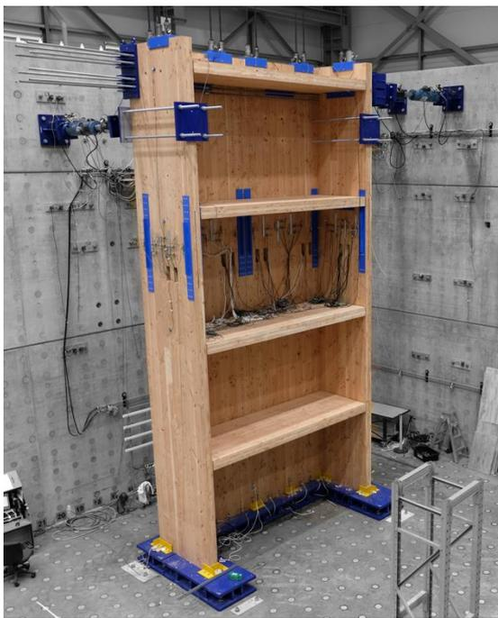
Fig. 1 - C-shaped core-wall specimen
