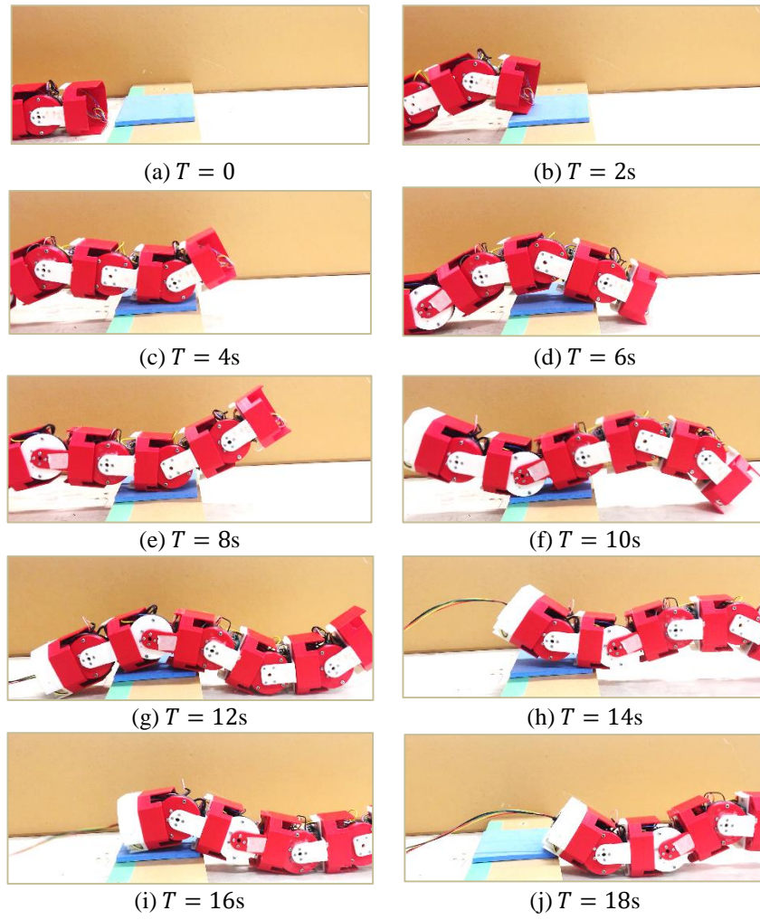
Fig. 15 The robot climbing over an obstacle
