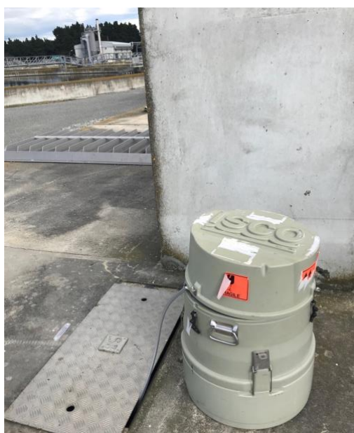
Figure 2-10. ISCO 3700 Autosampler with vinyl tubing onsite at Christchurch WWTP, positioned at the effluent sump.
