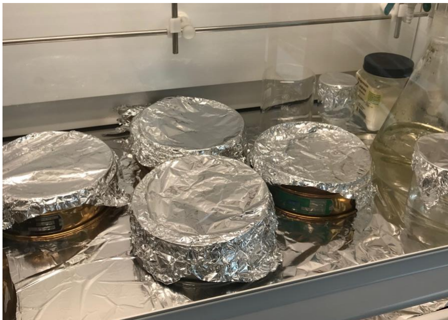
Figure 2-1. Aluminium foil-lined fumehood, with extraction equipment openings (sieves and beakers) covered with aluminium foil to reduce airborne microplastic contamination.
