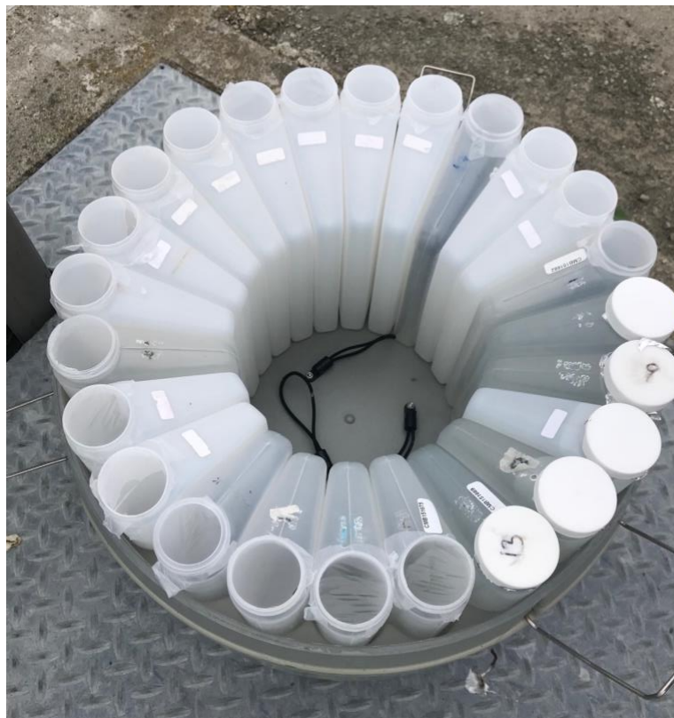
Figure 2-11. Polypropylene ISCO 3700 autosampler bottles in base of autosampler.
