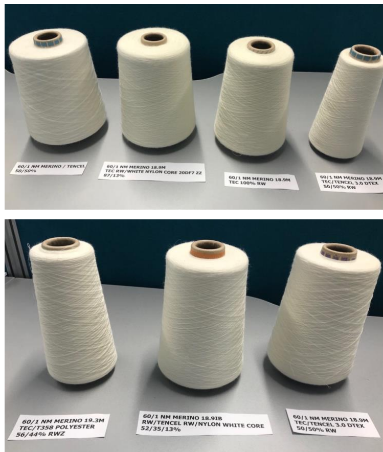
Figure 2-3. Merino/synthetic blend yarn spools. Top image, left to right: spool 7, spool 4, spool 5, spool 1. Bottom image, left to right: spool 2, spool 3, spool 6.
