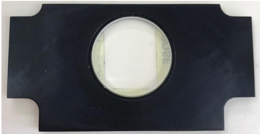
Figure 2-13. \text{CaF}_2 disk mounted onto a slide for FTIR analysis.
