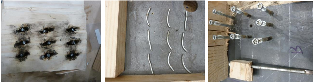
a) Timber embedment failure b) SFS dowel fatigue rupture in C-1 c) SFS dowels in B-1
