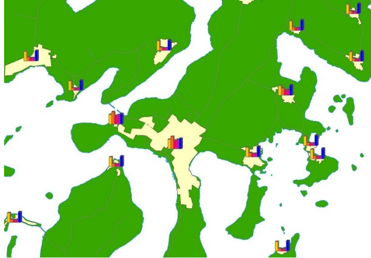
Figure 5.3. An example of output from the study of energy production methods for small communities in Tonga. The green shaded area is land and is surrounded by water (white). The relative sizes of communities (beige) and the prevalence of solar panels (yellow) wind of different strengths (orange, red and purple) and diesel generation (blue bar). From Jacobson and Brunton (2009).
