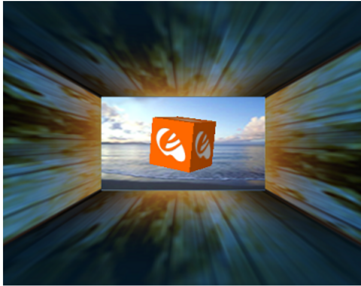
Figure 2.2: This virtual cube is used for training to control actions in the Emotiv Cognitiv suite. It floats about corresponding to detected actions and otherwise automatically returns to the middle of the screen.
