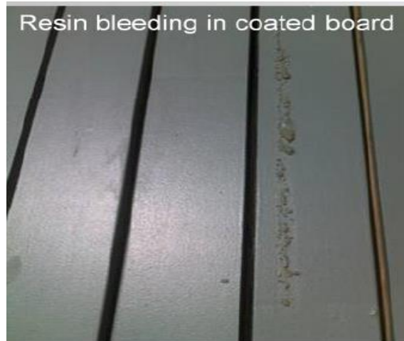
Figure 3: Resin dissolving paint on a board (photo credit: Solid Wood Initiative, New Zealand).
