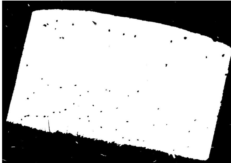
Figure 14: Image of a wood section in 8-bit format with threshold effect. These image enhancing features were applied in ImageJ software. Resin canals can be seen as black dots.
