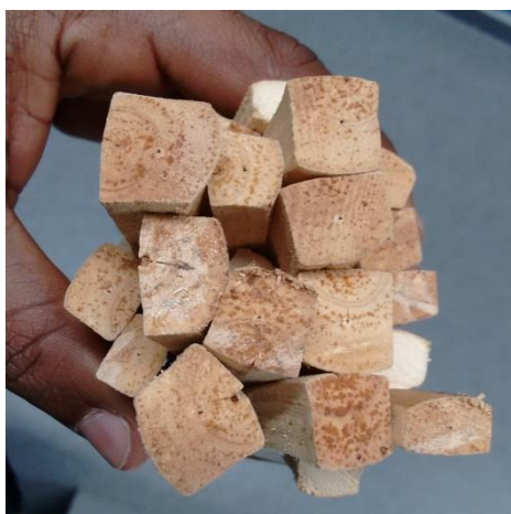
Figure 6: Cross-sectional ends of samples showing resin (the oily looking dots) after heating in an oven at 105° C for 24 h.
