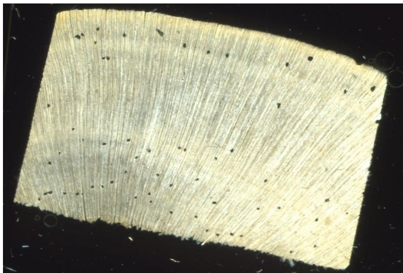
Figure 13: Image of a scanned wood section in polarised light displaying resin canals as black dots.
