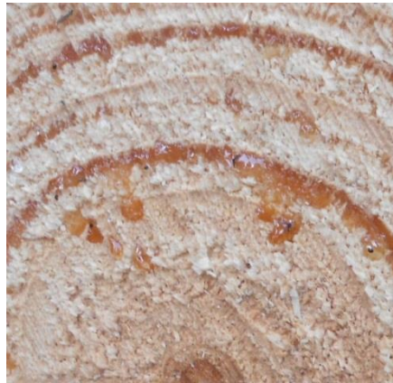
Figure 1: The cross-section of radiata pine wood with oil-looking resin.
