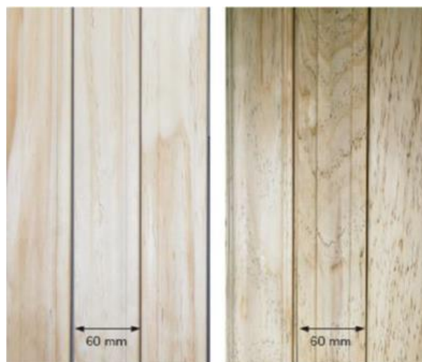
Figure 4: Variation in surface brightness between boards caused by resin canals. (photo credit: Solid Wood Initiative, New Zealand).
