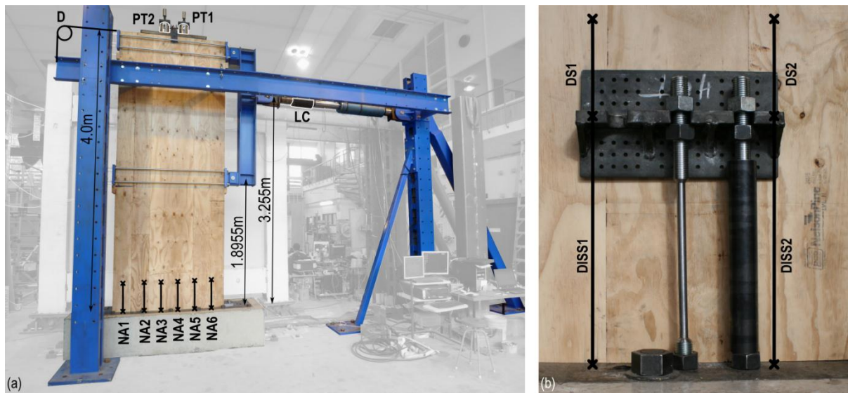
Figure 9. (a) Instrumentation setup for overall response and (b) instrumentation for detailing.
