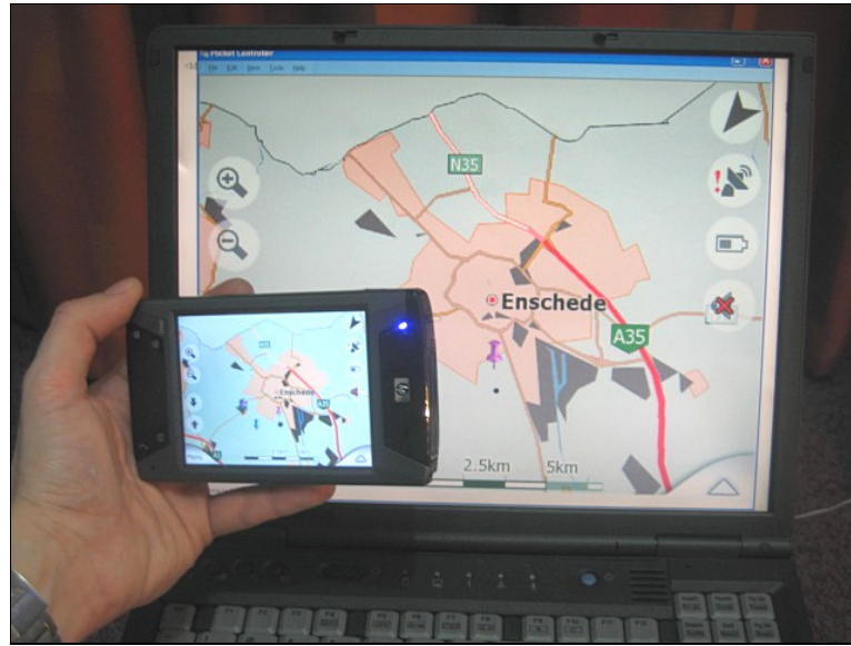
Figure 4.4 Remote PDA screen capture on the laptop via Wi-Fi connection
