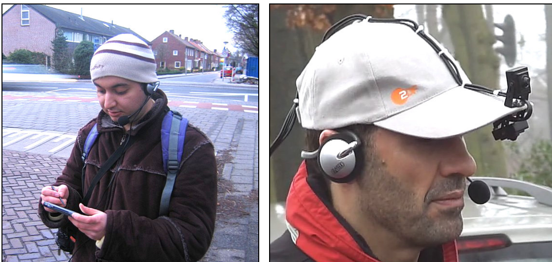
Figure 4.7 The wireless communication headset used in all the groups and the two cameras installed on the user's hat
