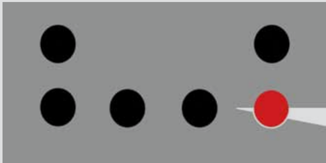
Corrosion-induced crack allowing water and air to bottom surface of corner strand
