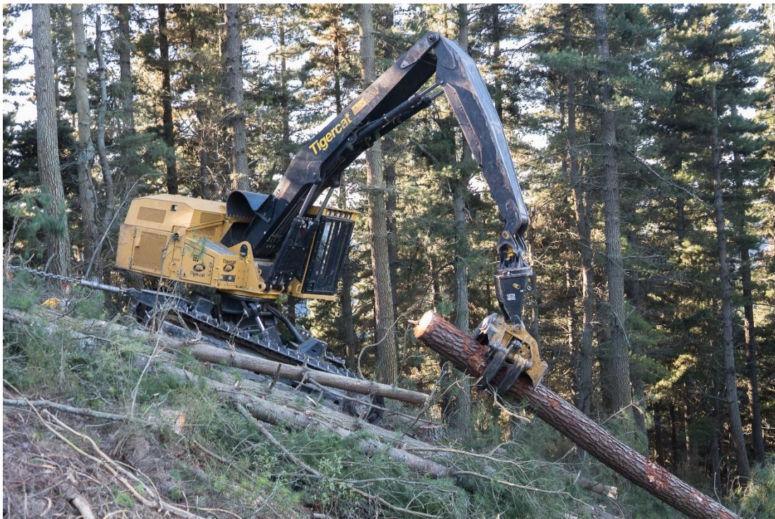
Figure 6.2 An example of a forest harvesting machine working on steep slope (photo courtesy of Phil Taylor)
